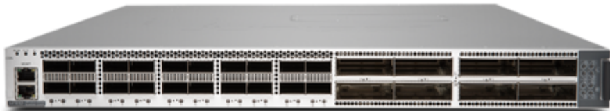
ACX6360 with 20 x QSFP28 and 8 x CFP2-DCO slots
